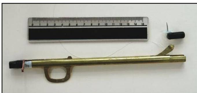
Figure 1. VEMCO V9 coded tag and tool designed to insert tag into mantle cavity.
